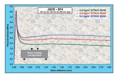
Note: These curves are based on averages of several beam tests. The toughness performance will depend on the concrete mix design used.
