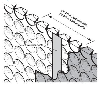
Hydroduct CF to be overlapped at all joints bonded centrally with Servitape
