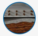
With PREPRUFE®, the membrane is fully sealed to the structural concrete and is unaffected by any ground settlement. The PREPRUFE® membrane remains fully bonded to the structure to resist hydrostatic pressure and avoid membrane stress.
