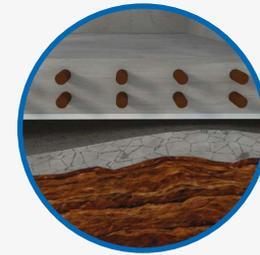
With PREPRUFE®, the membrane is fully sealed to the structural concrete and is unaffected by any ground settlement. The PREPRUFE® membrane remains fully bonded to the structure to resist hydrostatic pressure and avoid membrane stress.
