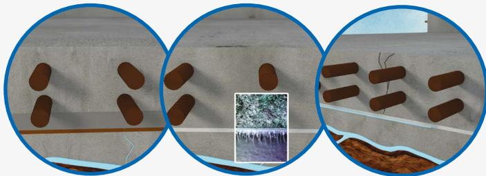
With PREPRUFE® membranes, the protection layer is eliminated and the membrane is bonded tightly to the structural concrete to prevent water penetration.
