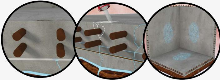
Conventional membranes are either unbonded or bonded to the substrate and normally covered with protective layers or screed separating them from the structure. When there is damage or a defect in the membrane, water can track between the membrane and the structural concrete looking for cracks or weakness in the concrete.
